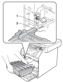
8 Turn the green lock lever (1) clockwise to the lock position.
